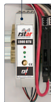
A flexDAQ enclosure shown with an open lid to reveal an installed RSTAR L900 RTU (on DIN rail), datalogger, radio and power supply.
