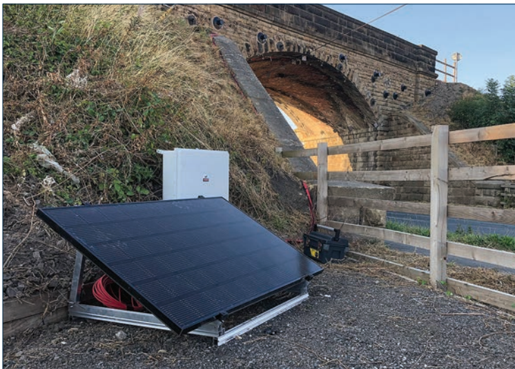
Data logger system shown with solar panel in foreground.
